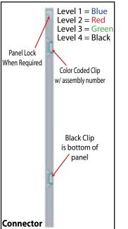
Each component has 2 clips, the lower clip is ALWAYS black. The top clip is color coded to distinguish the level. The color coded clip also contains the numbered label.
