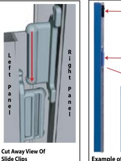
Components connect togetherCby aligning them and slidingfdownward connecting clipsvtogether.r
